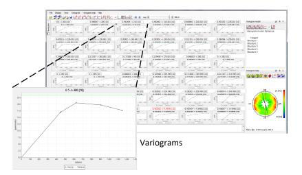
The geological model enables the grouping of materials of similar quality. A series of geostatistical tests are performed in order to define the parameter for the construction of a representative block model.
